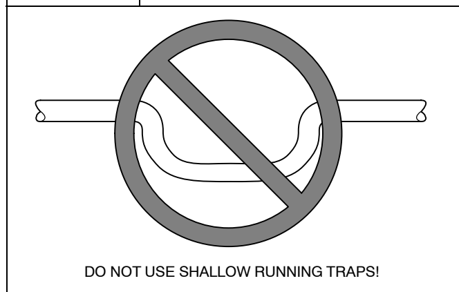
Figure 21 Insufficient Condensate Trap
